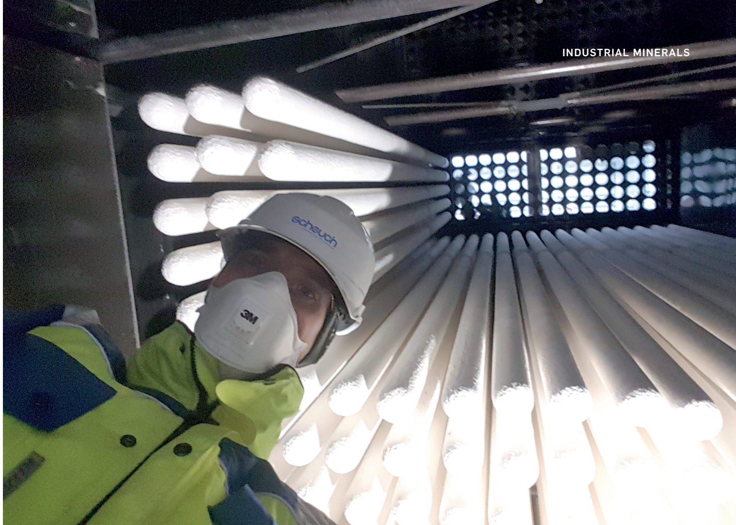
Long filter candles as the ideal solution in the cement industry.
