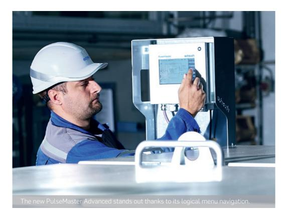
With the PulseMaster Advanced control unit. Scheuch is launching a new era of filter management. The new-generation device is fitted with a powerful processor and a touchscreen with full graphic display and user-friendly menu navigation. In order to avoid errors resulting from misunderstandings in a global workplace, there is a strong reliance on the use of representative symbols and images. The texts can easily be implemented in different languages at the request of the customer.
