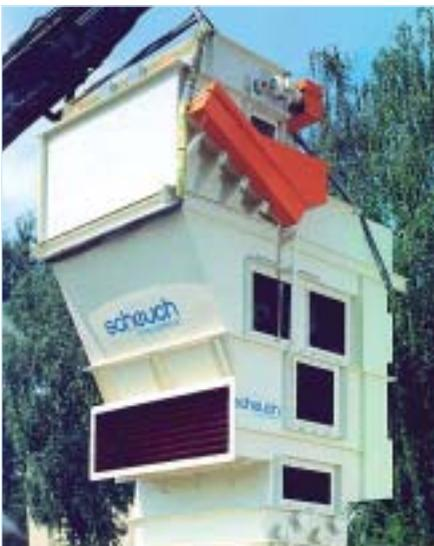
Scheuch first turned its attention to the topic of airstream sorting some 10 years ago and developed the SWSF fibre classifier (SWSF = Scheuch-Wind-Sichter für Fasern) for use in the production of MDF board. Its job is to clas-
